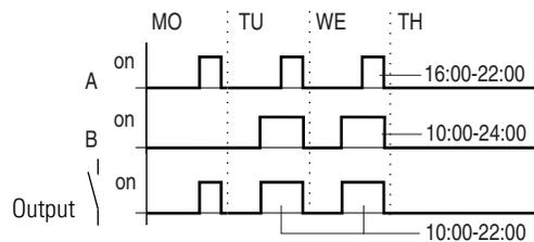
Turn-on and turn-off times always follow the channel which switches first.
