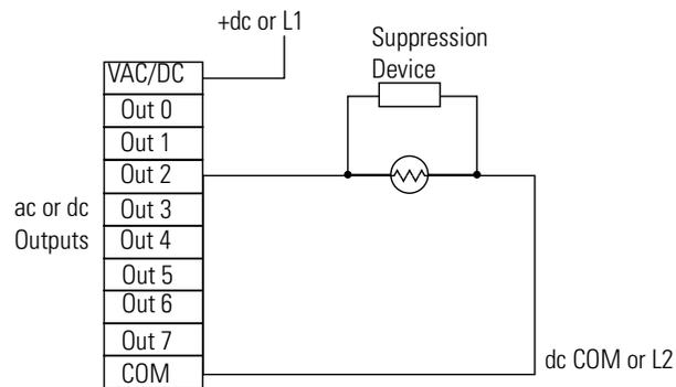
If the outputs are dc, we recommend that you use an 1N4004 diode for surge suppression, as shown below.
