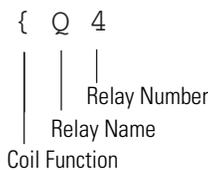
A relay is defined by its coil function, name and number.
