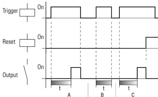
The trigger input starts the time (t). If the trigger input is disabled after the time has elapsed, timer is reset and the output is turned off (A). If the trigger coil drops out before the time has elapsed, the contact is not turned on (B). The reset coil has priority over the trigger coil and always resets the timer and turns the output off (C). If the preset is set to zero, the output follows immediately after the trigger signal.
