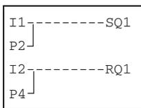
A lamp at output relay Q1 is turned on and off via inputs I1 and I2 or using cursor buttons up and down.
