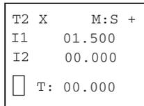
A timing relay is integrated into your circuit in the form of a contact. The function of the relay is defined via the parameter display. The relay is started via the trigger input TRG and can be reset via the reset input RES. A timer also resets when it is turned off. To prevent unpredictable switching states, use each coil of a relay only once in the circuit diagram.
