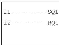
A self-latching circuit with wire break monitoring can alternatively be wired using the Set and Reset coil functions.
