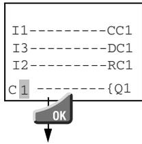
You can wire up coils RC1 and DC1 as required. Select relay contact C1, move the cursor to 1 and press Ok.
