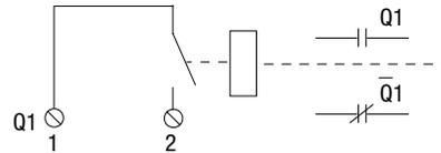
Outputs are controlled via the corresponding output relays:
