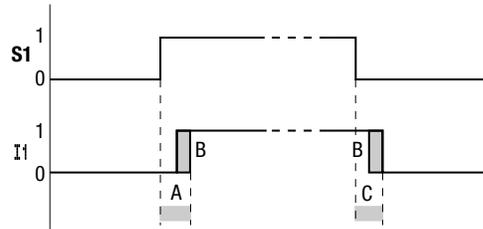
Typical delay times with the input debounce delay turned off are a few hundred  $\mu\text{s}$ , and are given in the specifications in Appendix A.
