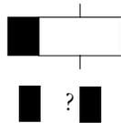
The relay switches a contact immediately and then resets it after the setpoint delay has elapsed. With random switching, the relay contact switches randomly at any time up to the specified time value (shown shaded in figure).
