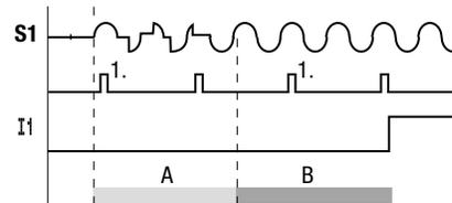
If a button or switch bounces (A), the delay time may be extended by 33 ms at 60 Hz (40 ms at 50 Hz) (A).
