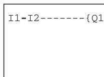
3. Press Esc to return to the Main Menu. A circuit diagram does not have to be completed before you can test parts of it with Pico.
