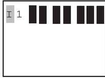
1. The first input contact is I1. Press Ok. Pico inserts the first contact I1 at the cursor position.
