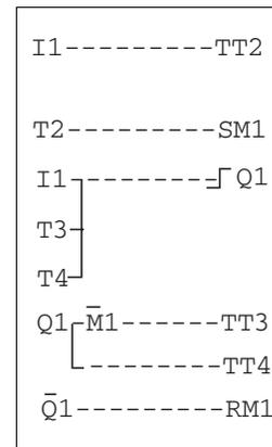
If you use Pico with a time switch, you can define both the stairwell lighting and the continuous lighting periods via the real time clock.
