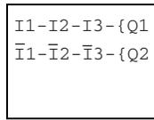
Q1 is controlled by a series circuit consisting of three make contacts (AND circuit).
