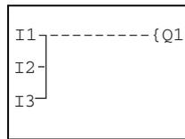
Q1 is controlled by a parallel circuit consisting of three make contacts (OR circuit).
