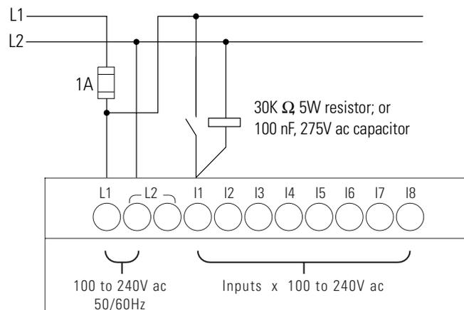
When using a 100 nF capacitor, the drop-off time of the input increases by 66.6 ms at 60 Hz (80 ms at 50 Hz). Also, a capacitor increases the amount of current seen by the input device. Do not use a bleeder capacitor in conjunction with reed switches.
