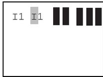
Again, Pico creates a contact I1 at the cursor. Change the contact number to I2 since break contact (normally closed) S2 is connected to input terminal I2.
