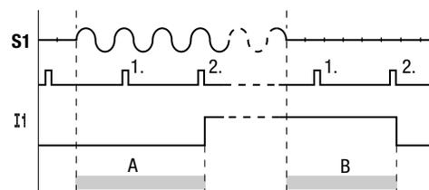
If the delay is switched on, Pico checks at 33 ms (40 ms for 50 Hz) intervals whether there is a half-wave present at an input terminal (1st and 2nd pulses in A). If Pico detects two pulses in succession, the device switches on the corresponding input internally.
