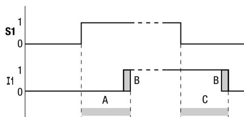
An input signal, S1, must be present at the input terminal for at least 20 ms before the switch contact will change from 0 to 1 (A) in the program. If applicable, this time must also include the program cycle time (B) since Pico does not detect the signal until the start of a cycle.
