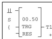
An automatic running light can be created by slightly modifying the shift register circuit. One output is always switched on. It starts at Q1, runs through to Q4 and then starts again at Q1. The marker relays for storage positions M1 to M4 are replaced by relays Q1 to Q4. The shift pulse I1 has been automated by the flasher relay T1. The cycle pulse M8 remains as it is.
