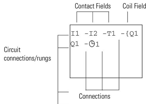
Connections are used to produce the electrical continuity between relay contacts and the coil. Connections can be created across several rungs. Each point of intersection is a connection. The circuit diagram display performs two functions:
