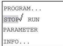
1. Switch to the main menu and select the RUN menu option (press Esc to go back to the Main Menu and use the arrow keys to highlight RUN).
