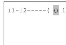
5. Press Ok. Then press Esc to leave the circuit diagram display. The diagram will be automatically saved.
