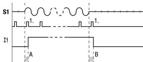
Pico switches the contact as soon as it detects a pulse (A). If no pulse is detected, Pico switches off the contact (B). The procedure for changing the delay times is described in Activate Debounce (Input Delay) on page 6-10.
