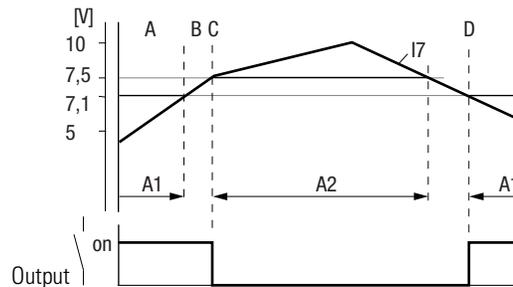
A1 sets relay output Q1 (A) up to a voltage of 7.1V. The hysteresis (B) is between 7.1V and 7.5V. At 7.5V, A2 causes the relay to reset (C). Q1 drops out and does not pick up again until A1 is set at 7.1V (D).
