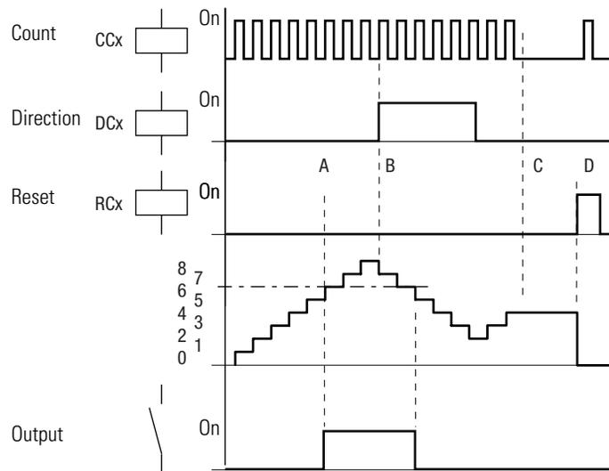
The relay contact of a counter with setpoint value 6 switches when the actual value is 6 (A). If the counting direction is reversed (B), the contact switches off when the actual value is 5. Without a counting pulse, the actual value is retained (C). The reset coil resets the counter to 0 (D).
