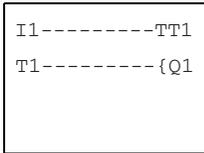
The on-delay can be used to gate short pulses or to initiate another movement after a time delay when a machine is started.
