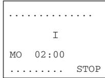
Press Ok to switch to the main menu. If there is an expansion module installed, the expansion module status screen is displayed. Press Ok again to switch to the main menu.
