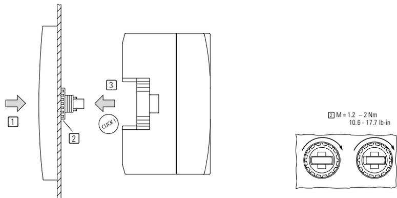
1. Insert the display unit through the mounting holes on the panel.
