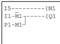
Input 'I1' is used to control output 'Q1'. Input I5 switches to Cursor button mode and deactivates circuit connection I1 via  $\bar{M}1$ .
