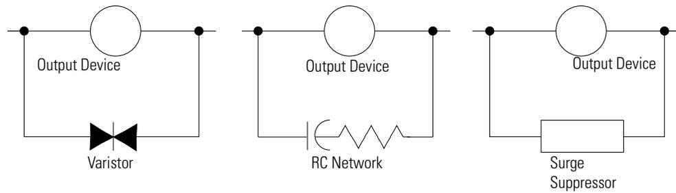
For inductive dc load devices, a diode is suitable. A 1N4004 diode is acceptable for most applications. A surge suppressor can also be used. See the table on page 2-14 for recommended suppressors.
