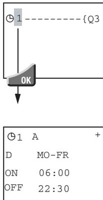
1. Enter the relay contact for the time switch in the contact field.
