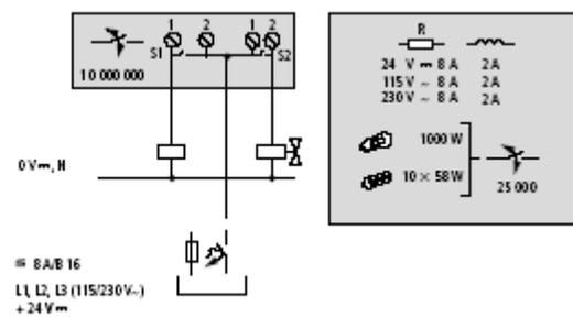
Unlike inputs, you can connect different phases to the outputs.
