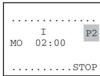
The Status menu display shows whether the P-Buttons are used in the circuit diagram.
