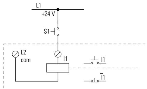
Connect devices such as buttons or switches to Pico input terminals.
