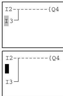
1. Position the cursor on the first contact field of a circuit connection.
