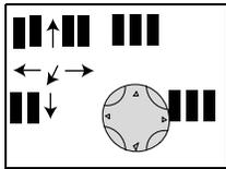
The wiring arrow works between contacts and relays. When you move the arrow onto a contact or relay coil, it changes back to the cursor and can be reactivated with Alt if required. Pico automatically wires adjacent contacts in a circuit connection up to the coil.
