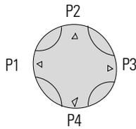
The buttons are contacts P1 to P4 in the circuit diagram. The P-Buttons can be activated and deactivated in the System menu.
