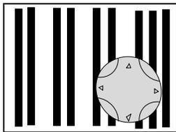
The first three double columns are contact fields and the right-hand triple column forms the coil field. Each line is a circuit connection. Pico adds the first contact automatically.
