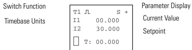
The coil terminals are not shown if you access the parameters via the PARAMETER menu option. The actual time is only displayed in Run mode. To view the actual time, call up the parameter display via the power flow display or using the PARAMETER option.
