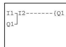
Latching circuits are used to switch machines on and off. The machine is turned on when the normally open push button connected to input terminal I1 is activated. The machine is turned off when the normally closed push button connected to I2 is activated.
