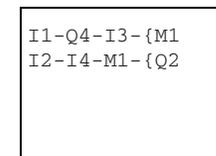
When wiring more than three contacts in series, use one of the marker relays.
