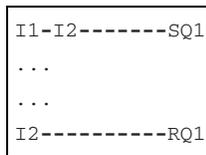
Use relay functions 'S' and 'R' only once per relay. If both coils are triggered at the same time, priority is given to the coil further down in the circuit diagram. This is shown in the preceding signal diagram in section 'B'.
