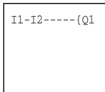
Switches S1 and S2 are wired to inputs I1 and I2. Relay K1 is represented by the relay coil {Q1. The symbol “{” identifies the coil's function, in this case a relay coil acting as a contactor. Q1 is one of up to six Pico output relays.
