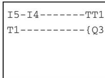
You integrate a timing relay into your circuit in the form of a contact and coil.
