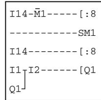
As long as  $I14 = 1$ , the remaining circuit diagram is skipped. If  $I14 = 0$ , the circuit diagram is processed. If the expansion module drops out for any reason, the circuit diagram is skipped.  $M1$  detects whether the circuit diagram was processed for at least one cycle after the power supply switched on. If the circuit diagram is skipped, all the outputs retain their previous state. The next example should be used if this is not desired.
