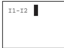
5. Press Ok to move the cursor to the third contact field. You do not need a third relay contact, so you can now wire the contacts directly to the coil field.
