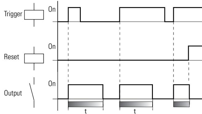
The reset coil has priority over the trigger coil and resets the relay contact before the time has elapsed. If the time is set to zero, the contact is set for the duration of one program scan.
