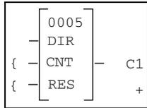
The maximum counter frequency depends on the length of the circuit diagram in Pico. The number of contacts, coils and circuit connections used determines the scan time (cycle time) required to process the Pico circuit diagram.
